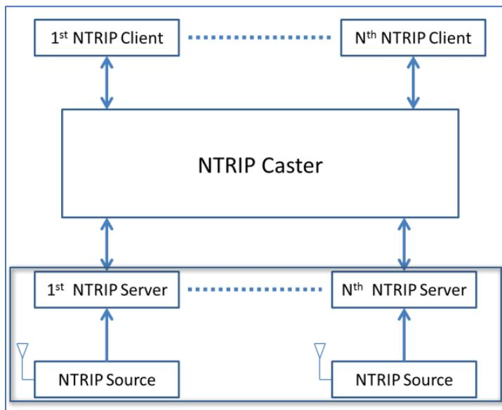
Normally the Ntrip Source and Ntrip Server are integrated into the GNSS receiver, basically we call it [Base/Reference Station]. Ntrip Caster is normally a software running on the computer. And Ntrip Client is normally called [Rover].
