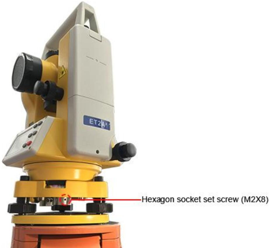
6. Repeat step 5 until the laser spot entirely coincides with the cross target when rotating the instrument in any direction.
