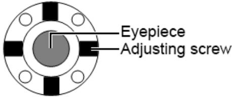
11. Repeat the whole process of checking and adjusting the collimation error until the error is less than or equal to 8".
