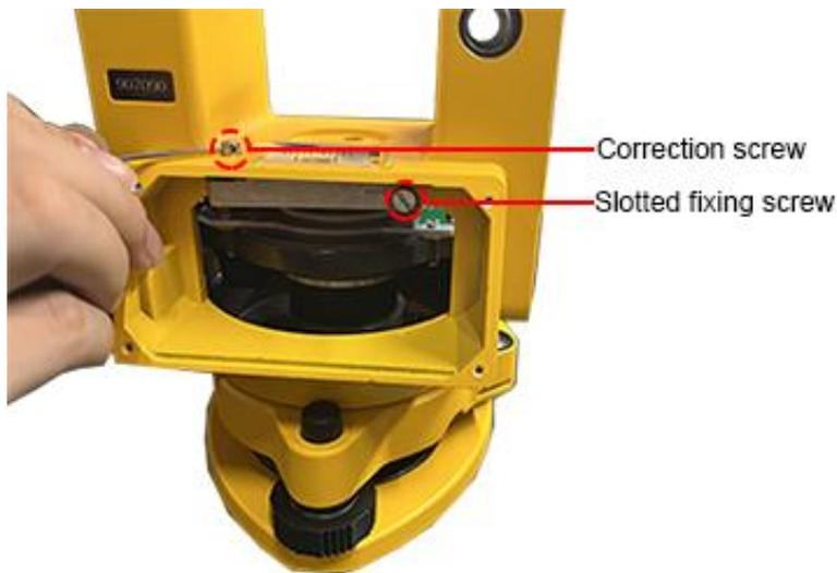
2. Unscrew the slotted fixing screw of plate level with slotted screwdriver, take down the slotted fixing screw.
