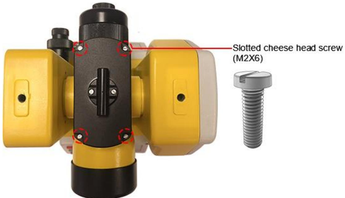
4. To make the laser spot coincide with the target center, adjust the four adjusting screws:
