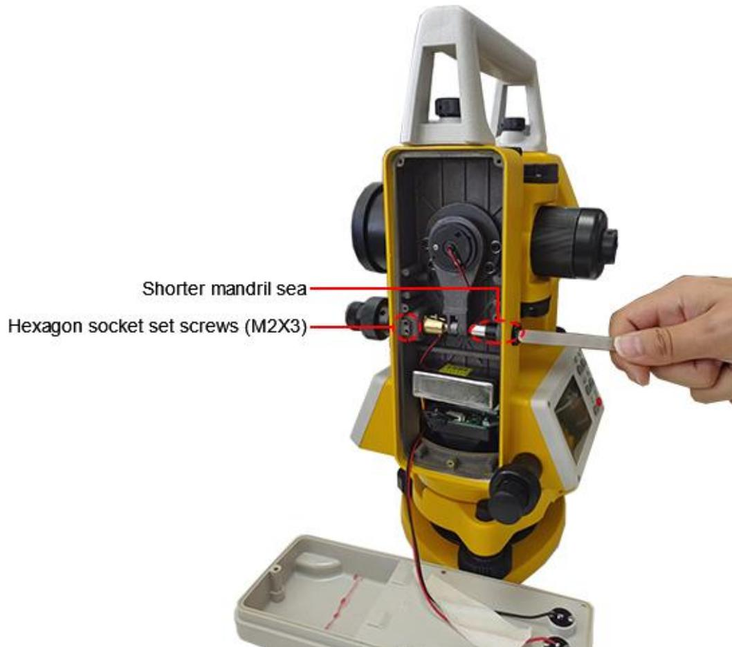
2. Loosen the two hexagon socket set screws (M2X3).
