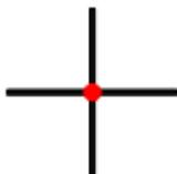
4. Rotate the instrument, and observe if the bubble and the laser spot still coincides with the cross target:
