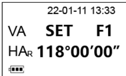
9. Aim at the reticle of collimator or the obvious target at a distance, and press **OSET**:
