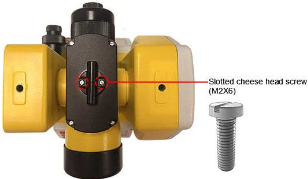
5. Fix the tightening screws, and make sure the optical sight collimates the mark.
