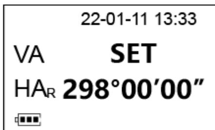
12. Repeat the whole process of checking and adjusting the vertical index error until the error is less than or equal to 10".
