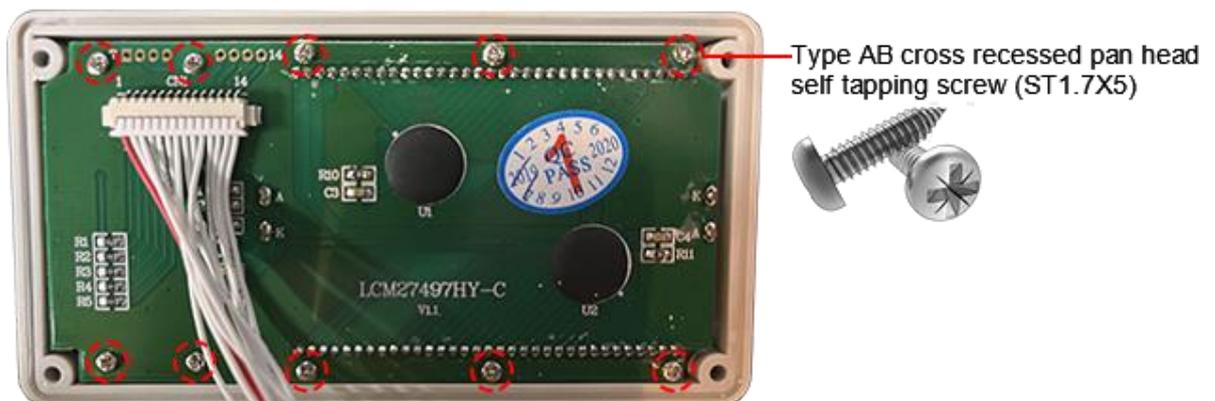
2. Remove the LCD module:
