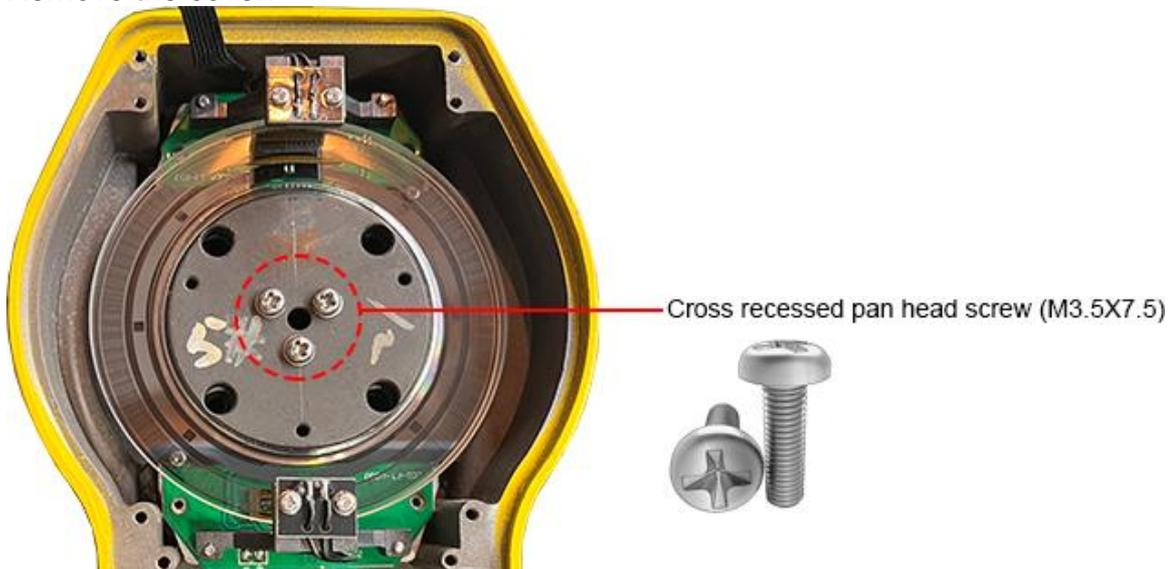
3. Remove three cross recessed pan head screws (M3.5X7.5) that fix the vertical circle, and remove the vertical circle:
