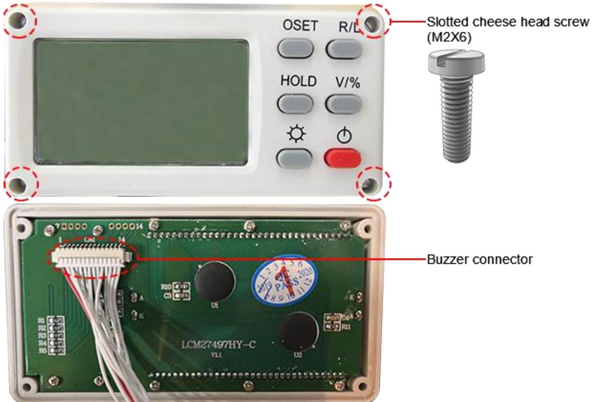
To disassemble the display, do the following:
