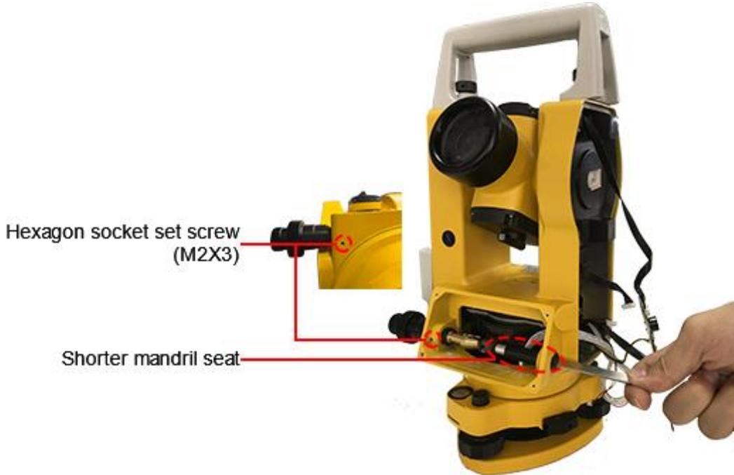
2. Loosen the two hexagon socket set screws (M2X3):
