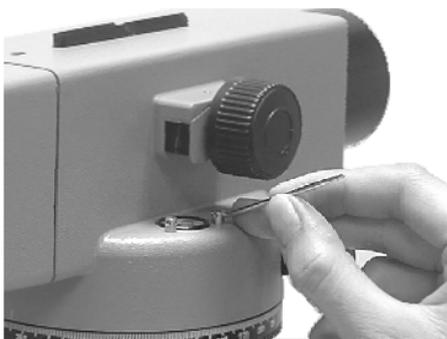
Fig.5 Adjusting the circular bubble.
